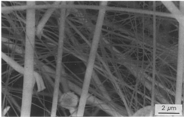
Figure 12 \text{Si}_3\text{N}_4 whiskers obtained using nickel impurity.
